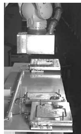
Component transport using a vacuum pickup
