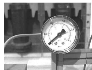
Pressure gauge for measuring the air pressure
